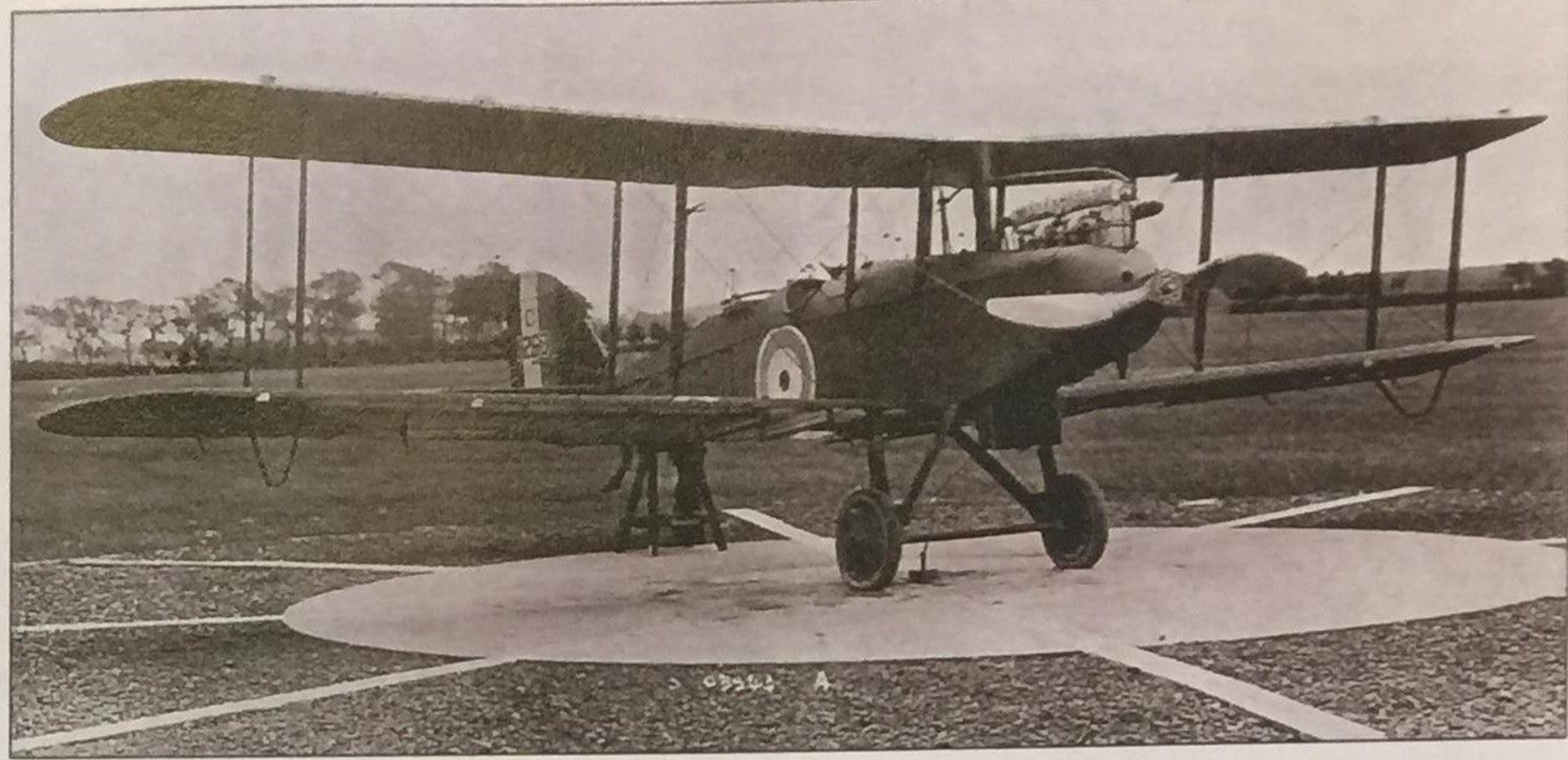
ABOVE Airco D.H.9 C1263, built by G. & J. Weir of Glasgow, has its compass swung on the compass base at Renfrew in 1918.
